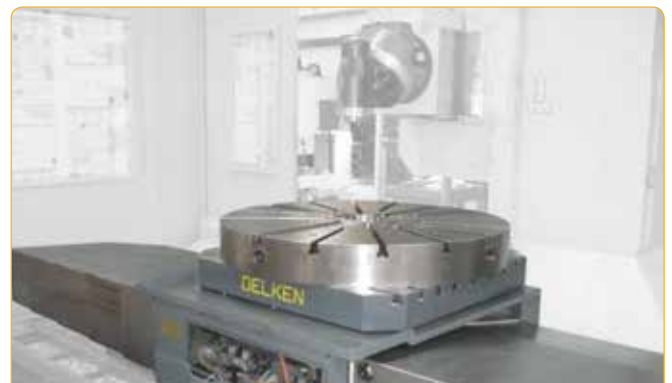
Milling roto-translating table, 1200x1200 – X2500 – 7 Ton., matched to a milling machine. Working of general machineries
