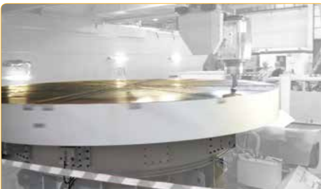
Turning and milling rotary table, Ø 4000 – 20 Ton. – 80 Rpm, matched to a portal milling machine. Working of details of military sectors
