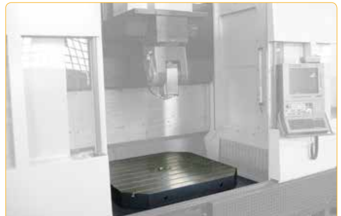
Milling rotary table, 2000x2000 – 12 Ton., matched to a vertical milling center Working of moulds
