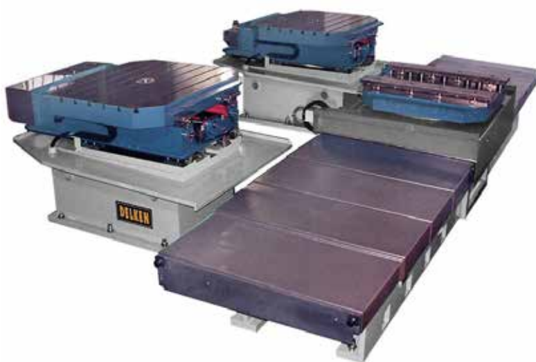
NC Milling roto-translating complete with palletized system Pallet 1000x1200 – Translation stroke X 2500 mm – Capacity 7 Ton
