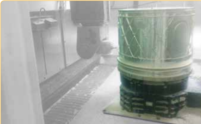
Turning and milling torque table, Ø 1000 – 3 Ton. – 300 rpm Matched to portal milling Working of aeronautical details
